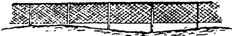
TOP RAIL STRAIGHT — Leaves spaces beneath fence if ground is not straight.
