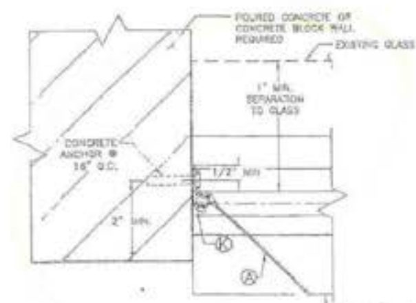
END CONNECTION DETAIL ⑤
