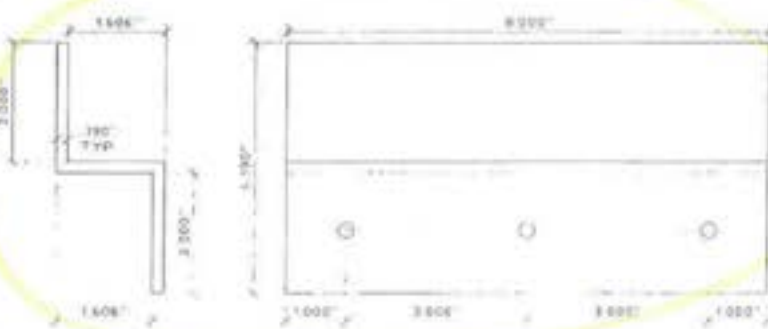
10. "2" BAR - PROFILE & LAYOUT SCALE: HALF SIZE
