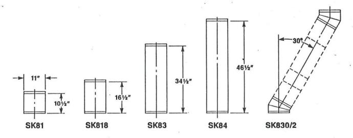
NOTE: THE INSTALLED LENGTH OF ANY CHIMNEY SECTION IS 1" LESS THAN ITS TOTAL LENGTH, EXCEPT FOR THE LAST SECTION INSTALLED.
