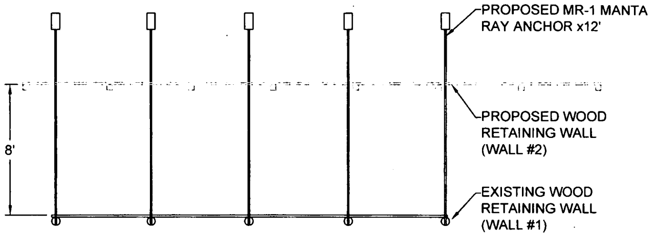
SECTION 1 PROPOSED MANTA RAY ANCHORS TO EXISTING WALL - WALL #1 DETAILED PLAN VIEW SCALE 1" = 6'
