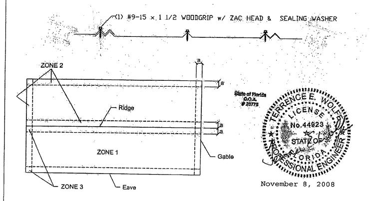
Note: Dimension (a) is defined as 10% of the minimum width of the building or 40% of the mean helght of the roof, whichever is smaller, however, (a) cannot be less than either 4% of the minimum width of the building or 3 feet.
