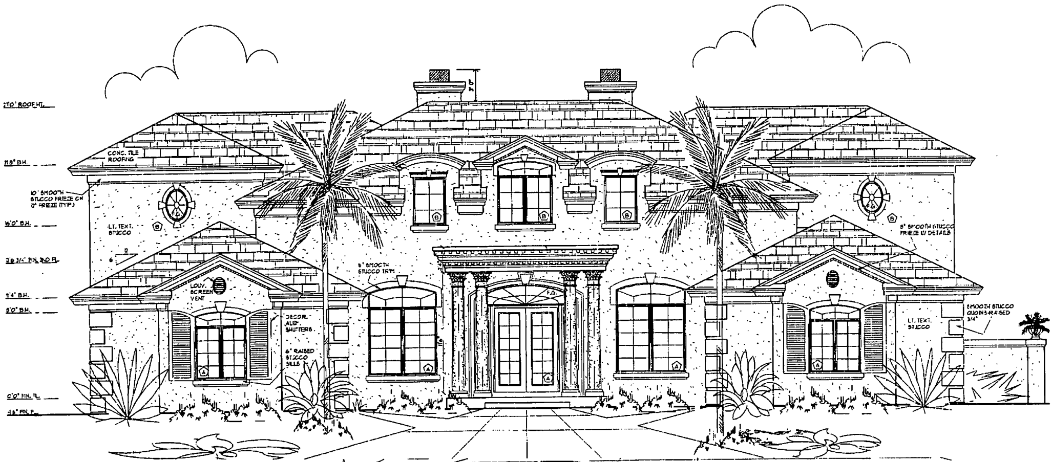
Front Elevation - 2 ft. Chimney - 1 ft. Spark Arrestor
